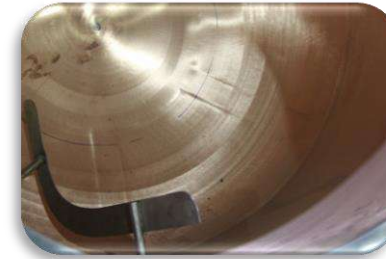
AISI 304 Quality stainless mixing pallets
