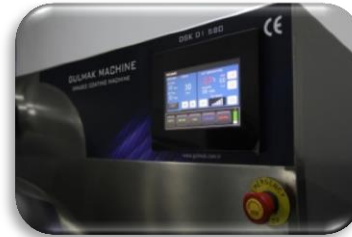
Touch control panel
